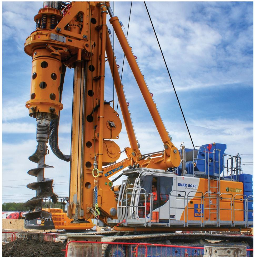
For example, the 183No piles required for the TBM Launch Pit (Phase I) was an increase on an original scope of 120No piles; the TBM Launch Pit was increased in length to aid later construction of a syphon for the Werrington Brook that passed through the site. Piling was also expected to be wet, however Bauer quickly discovered that the piles were dry and that the BG45 drilling rig had more than enough torque to drill the strong Cornbrash Limestone, which was encountered at 11m to 13m depth.
